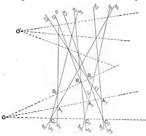
Therefore the lines joining their vertices are concurrent; that is, the lines joining the points  $b_2b_3$ ,  $b_3b_1$ ,  $b_1b_2$  respectively to the points  $c_2c_3$ ,  $c_3c_1$ ,  $c_1c_2$  are concurrent.
